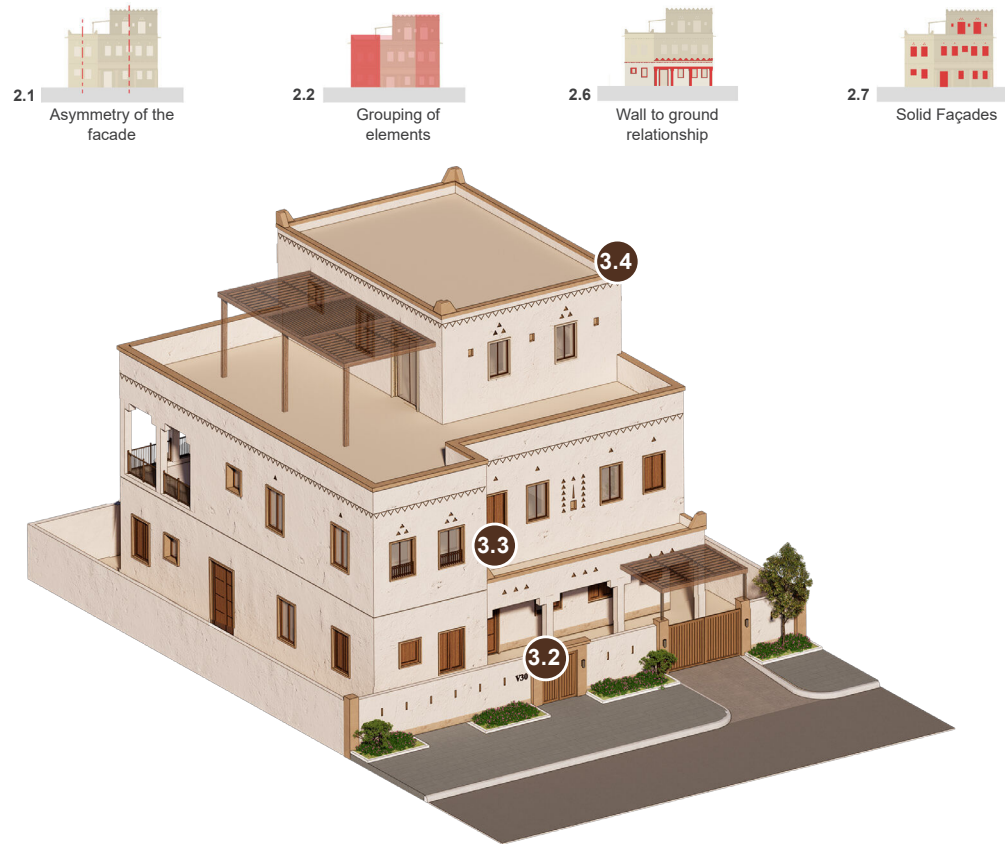
Axonometric view showcasing an example of the application of compositional rules for transitional style residential villa.
