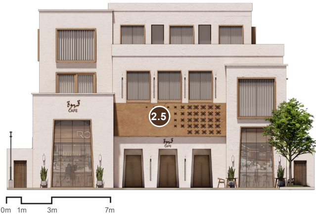
Elevation view showcasing an example of the application of compositional rules for contemporary style low-rise mixed-use buildings.
