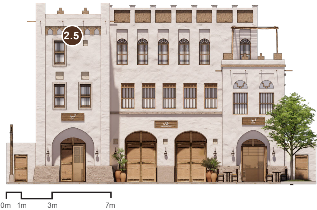
Elevation view showcasing an example of the application of compositional rules for traditional style low-rise mixed-use buildings.
