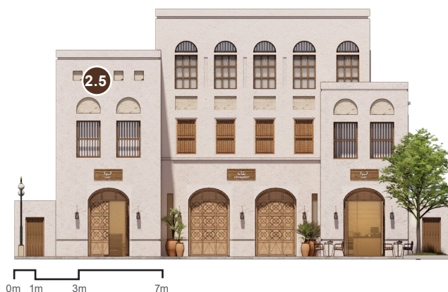
Elevation view showcasing an example of the application of compositional rules for transitional style low-rise mixed-use buildings.
